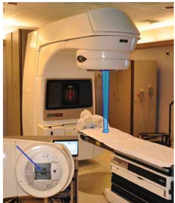
Figure 2. A 6-18MV conventional linear accelerator at Lancaster General Cancer Center. The linear accelerator directs high energy photons in a step and shoot fashion towards a target as demonstrated by the blue beam. At bottom left is a close up view of the multi-leaf collimator (MLC, blue arrow) which resides in the head of the machine. The leaves of an MLC shape the beam. In IMRT, the leaves continuously move in complex geometric patterns to modulate the intensity of the beam. This results in highly conformal distributions of radiation dose.
